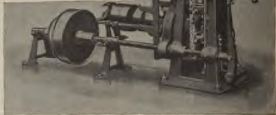
FIG. 11212. SHOWS NO. 2 MACHINE AND COUNTERSHAFT.
